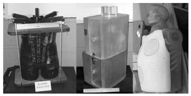
Figure 1-1. Examples of Phantoms Used in Radiation Measurements
