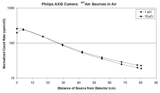
Figure 1-21. Normalized Count Rates in AXIS Camera from <sup>241</sup>Am Sources in Air
