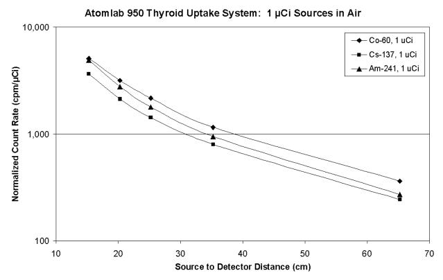
Figure 1-26. Normalized Count Rates in Atomlab 950 Thyroid Uptake System from 1 µCi Sources in Air
