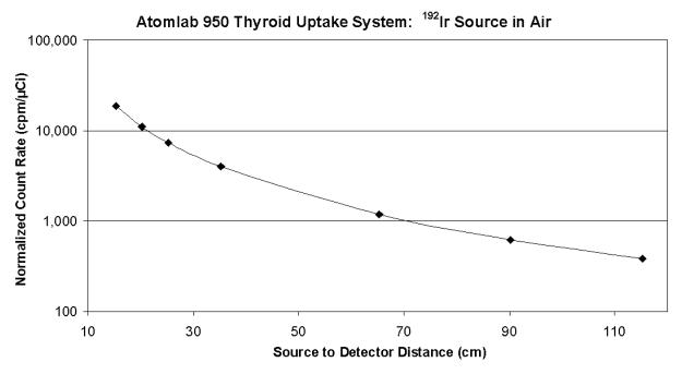
Figure 1-27. Normalized Count Rates in Atomlab 950 Thyroid Uptake System from  $18 \ \mu Ci^{192}$ Ir Source
