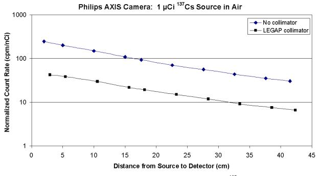
Figure 1-20. Normalized Count Rates in AXIS Camera from <sup>137</sup>Cs Source in Air
