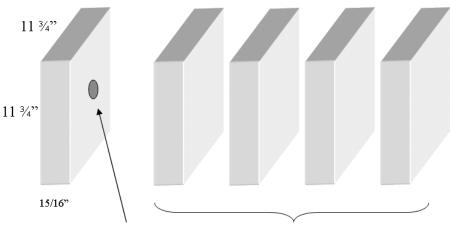
Disk- source mounting holeAcrylic slabs (1 to 10)Figure 1-2. Acrylic Phantom:Schematic View of Components
