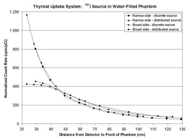
Figure 1-32. Count Rates in Atomlab 950 Thyroid Uptake System from Discrete and Distributed <sup>131</sup>I Sources
