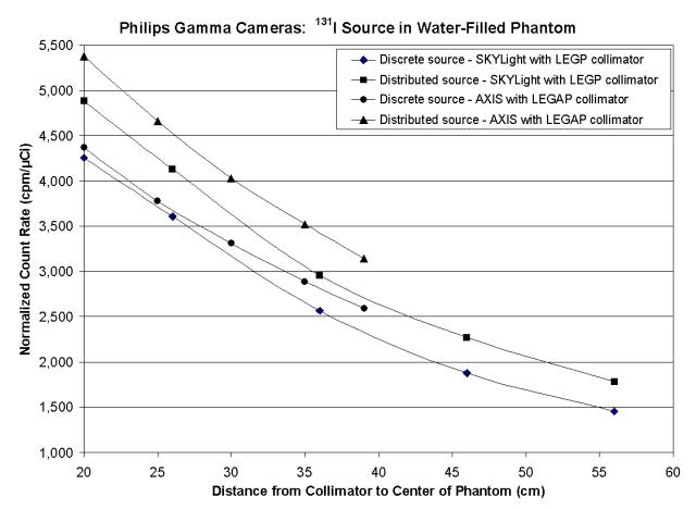
Figure 1-31. Count Rates in Philips Gamma Cameras from Discrete and Distributed <sup>131</sup>I Sources
