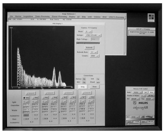
Figure 1-12. PHA Screen on AXIS Camera Display Console, Showing <sup>60</sup>Co Spectrum
