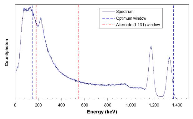
Figure 2-8. Pulse Height Spectrum of <sup>60</sup>Co Distributed in Lungs, Showing Energy Windows
