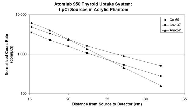
Figure 1-28. Normalized Count Rates in Atomlab 950 Thyroid Uptake System from 1 µCi Sources in Acrylic Phantom
