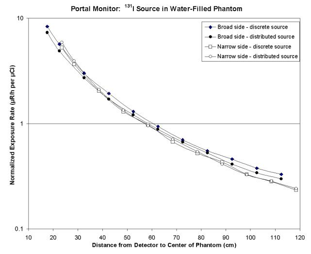
Figure 1-33. Exposure Rates on Waste Monitor from Discrete and Distributed <sup>131</sup>I Sources
