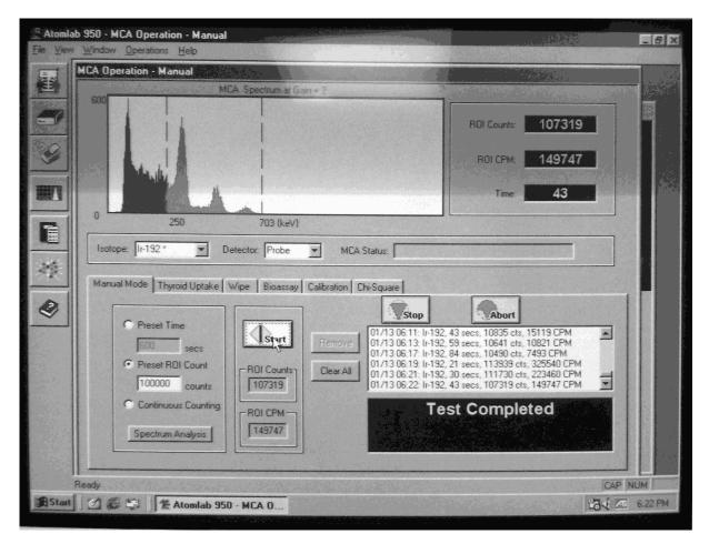
Figure 1-14. Atomlab 950 MCA Screen Showing Highlighted Region with <sup>192</sup>Ir Photopeaks
