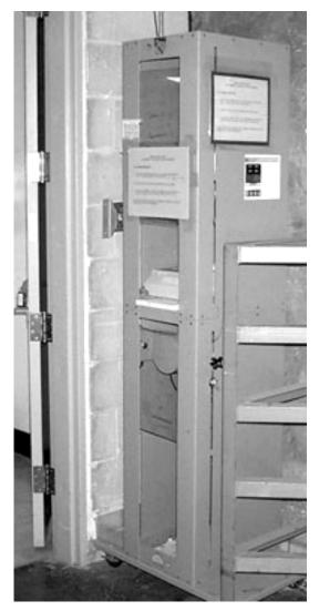
Figure 1-16. Detector Assembly of the HMC Waste Monitor
