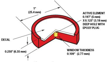
Figure 1-5. <sup>137</sup>Cs and <sup>60</sup>Co Sources (IPL 2003)
