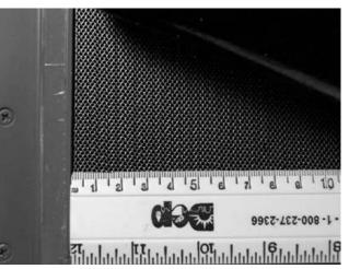
Figure 1-11. Back of Collimator Showing Corrugated Lead Strips
