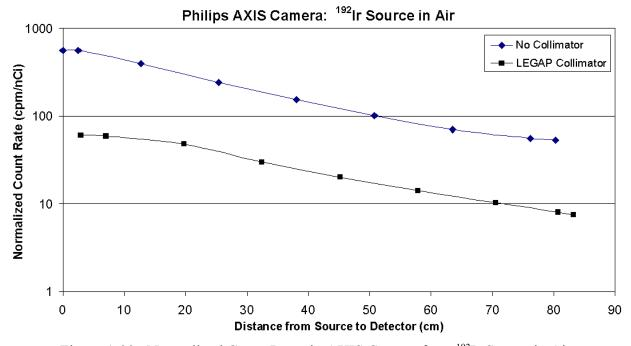
Figure 1-22. Normalized Count Rates in AXIS Camera from <sup>192</sup>Ir Source in Air
