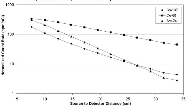
Philips AXIS Camera, No Collimator: 1 µCi Sources in Phantom
