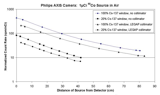
Figure 1-19. Normalized Count Rates in AXIS Camera from <sup>60</sup>Co Source in Air
