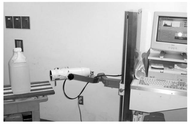
Figure 1-13. Atomlab 950 Thyroid Uptake System
