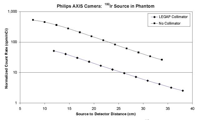
Figure 1-25. Normalized Count Rates in AXIS Camera from 18 µCi <sup>192</sup>Ir Source in Phantom
